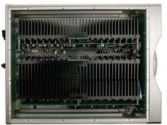
Massive heatsinking required for class A power amp
