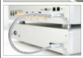
Above: Evolution Two inputs labelled only as S1-4. B1-3 and C1-3 on the panel (single-ended/balanced/CAST), but can be assigned pre-set names for the fluorescent display like 8TRK, DCC, GAME and HI-8; [left] unlike power amp, power connection from PSU to pre-amp is by cable
