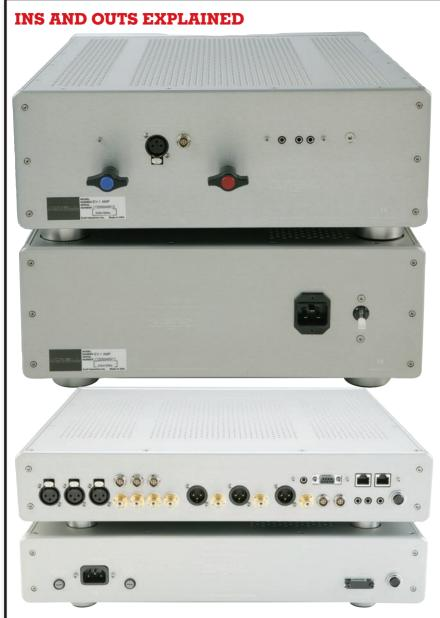
power amp includes XLR and CAST input [Below] Evolution Two pre-amp includes RS-232, RJ-45 and 3.5mm jacks, the latter for multiroom control
